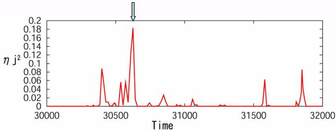
The above figure shows the time evolution of the volume integrated Joule heating rate. The arrow indicates the time when the largest magnetic reconnection takes place.
