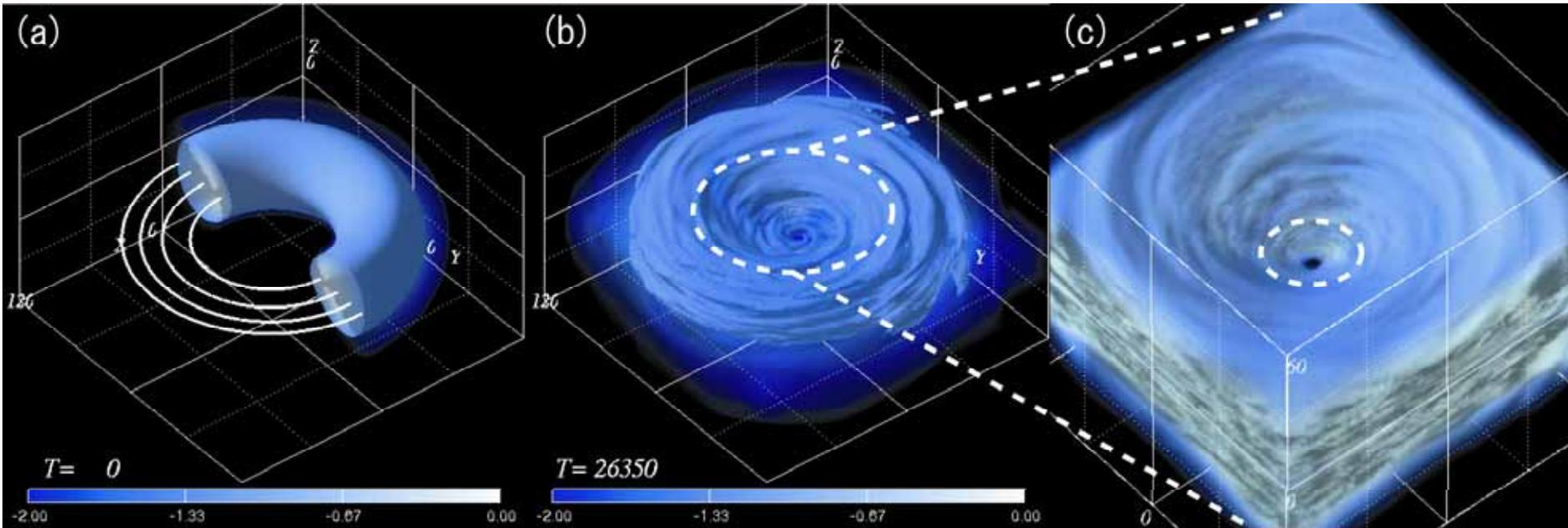
The equilibrium torus threaded by weak toroidal magnetic fields ( $\beta = 100$ ). Magnetic fields are amplified due to the magneto-rotational instability and saturates when plasma  $\beta$  is about 10. The MHD turbulence driven by MRI enhances the angular momentum transport rate and enables mass accretion.
